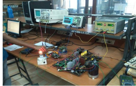
Figure 9: Experimental set-up of the solar inverter module
