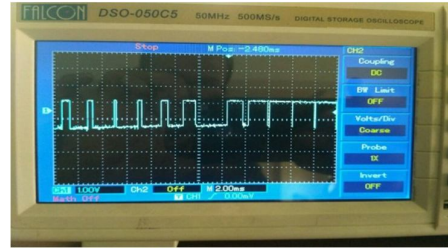
Figure 11: The PWM wave generated at pin No.9 of the DSP
